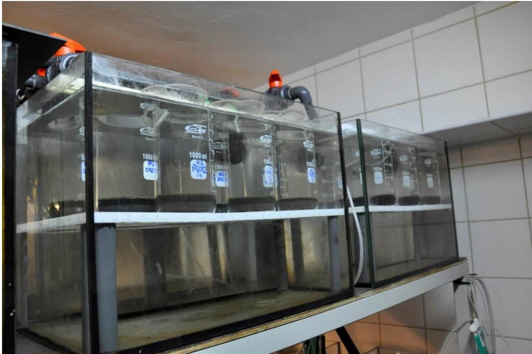
Fig. 17. The set-up of the experimental system for sediment toxicity testing.
